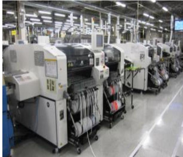
SMT process: mounting the parts
